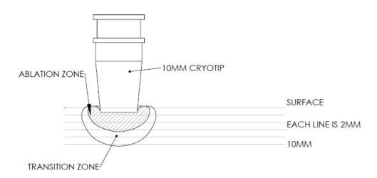
CROSSHATCHED AREA IS THE ABLATION ZONE ABLATION ZONE IS COLDER THAN -20\*C TRANSISTION ZONE IS BETWEEN 0\*C AND -20\*C BASED ON FREEZING OF BALLISTIC GELATIN c.) Expected Cryoablation zone for 19mm Tip (data derived from bench testing on ballistic gelatin)
